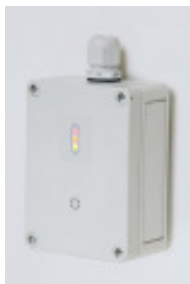
IP65 plastic enclosure with LED indicators Power supply = Green Low-Alarm = Yellow High-Alarm = Red
